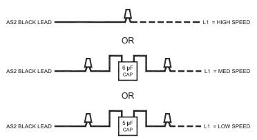
NOTE: A 2.5  $\mu\text{F}$  CAPACITOR IS ALWAYS USED ON THE 120 VAC "N" LEAD, AND IS WIRED BETWEEN THE WHITE AND BROWN LEADS OF THE MOTOR.
