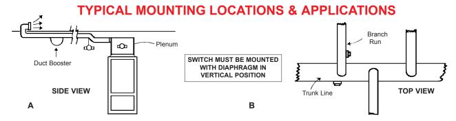
Switch activates Duct Booster by sensing positive pressure on either plenum, trunk, or branch lines as shown in Figures A and B above.
